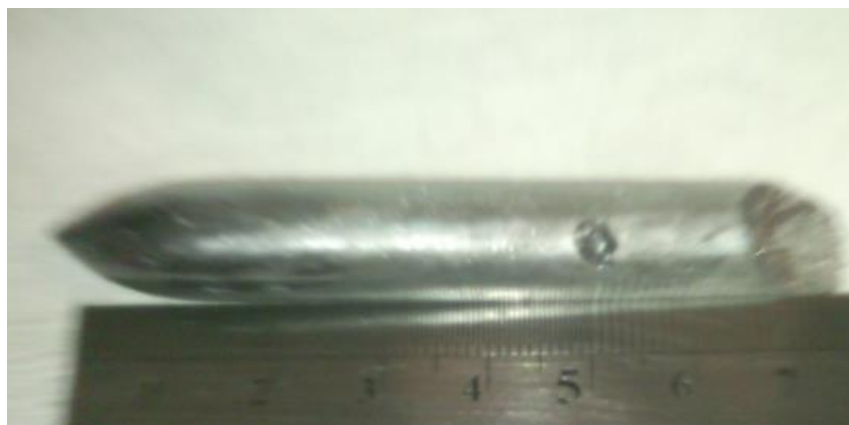
Figure 4: Synthesized material and grown crystals of InSe:Zn
