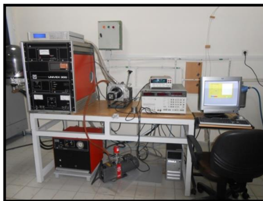
Figure 1The experimental setup where the I-V-T and C-V-T measurements
